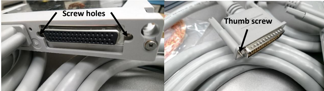
Left: Rear view of terminal block showing the plastic surrounding the connector. Right: Fifty-pin, D-sub connector with short thumb screws
